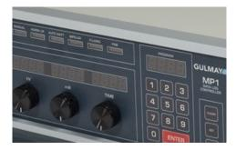
**The Gulmay MP1 analogue controller** is a microprocessor based controller designed for use with Gulmay high voltage X-ray generators. Available as a 19 inch rack-mount unit or in a desktop housing, the MP1 is factory programmed for use with over 110 X-ray tubes.
